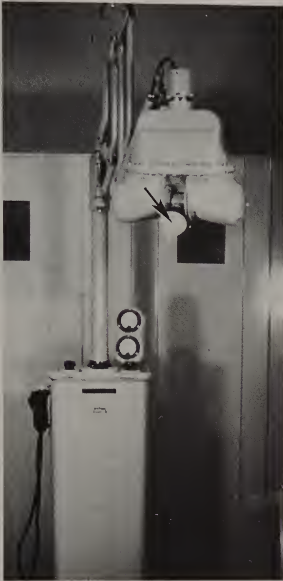
Figure 13.8 Short, Plastic Pointed BID. Short, plastic pointed BID (arrow) on vintage x-ray machine.
