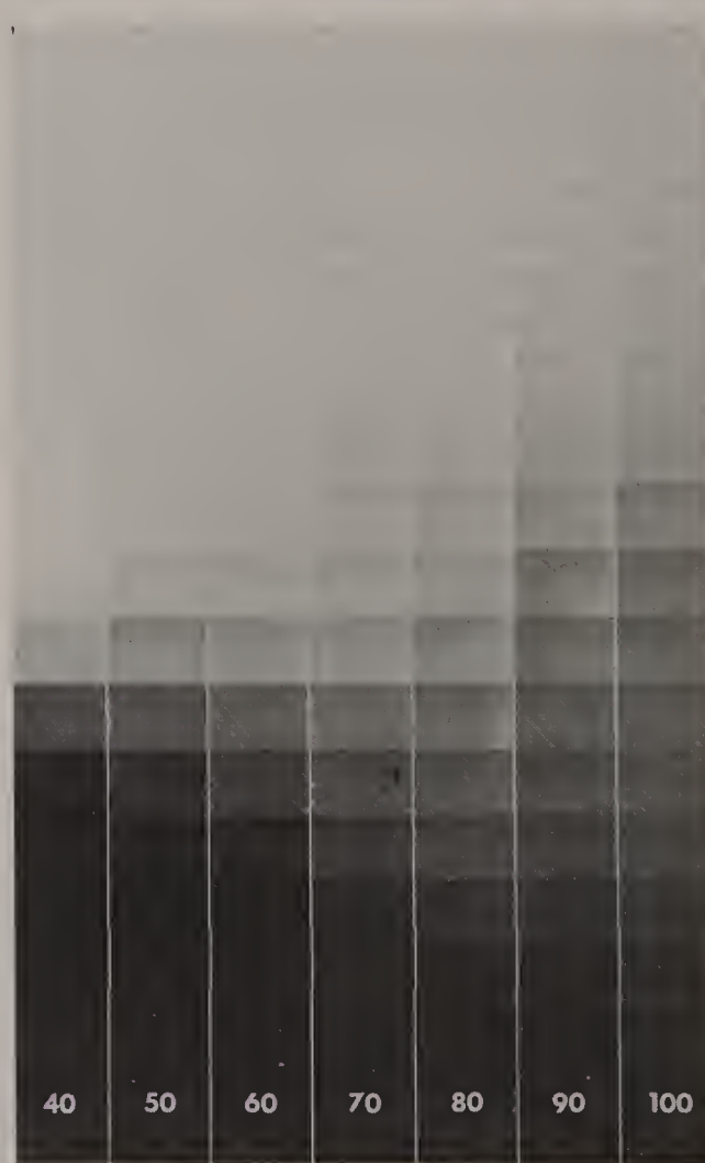
Figure 3.4 Contrast by Penetrometer. Comparison of long-scale and short-scale contrast using penetrometer.
