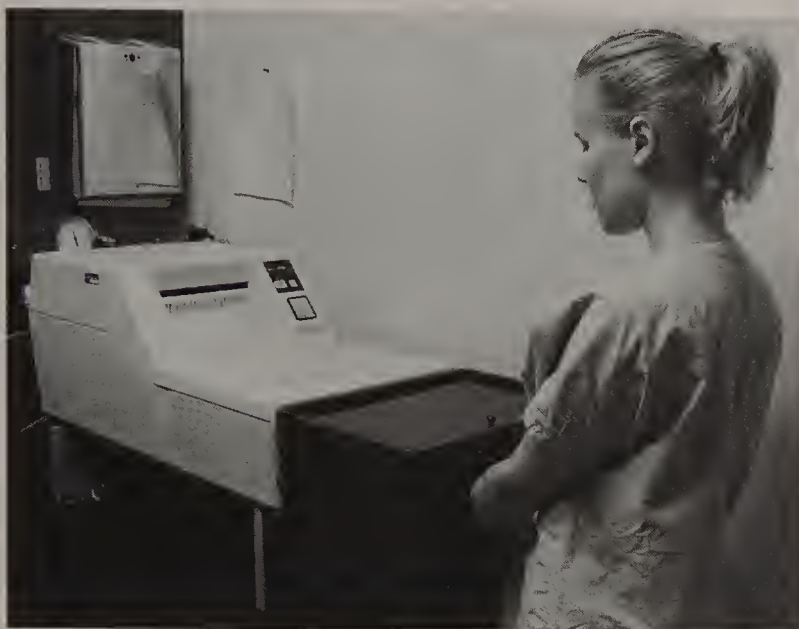
Figure 6.11 DENT-X 9000 Automatic X-Ray Film Processor. Dent-X 9000 with a daylight loader. It features a unique replenishing system that controls all processing chemistry. Infrared sensors measure film size on input and replenish (refresher) developing and fixing solutions based on the amount of film being processed. Develops all sizes of film up to 8 \times 10 -inch size. Dry films in 4.5 minutes, and endo wet readings in 1 minute. (Courtesy of Dent-X Co., Elmsford, NY 10523).
