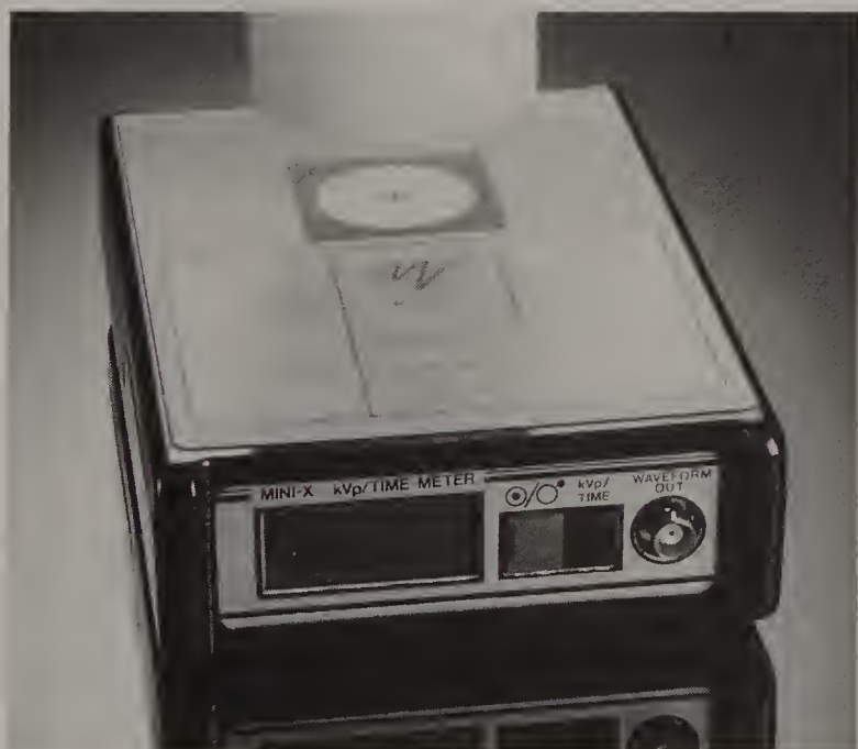
Figure 8.6 Checking the Accuracy of the kVp Setting. The kVp meter used to check kVp setting accuracy; the BID is aimed at the target area on top of the device. This kVp meter also measures exposure time to check the timer switch.
