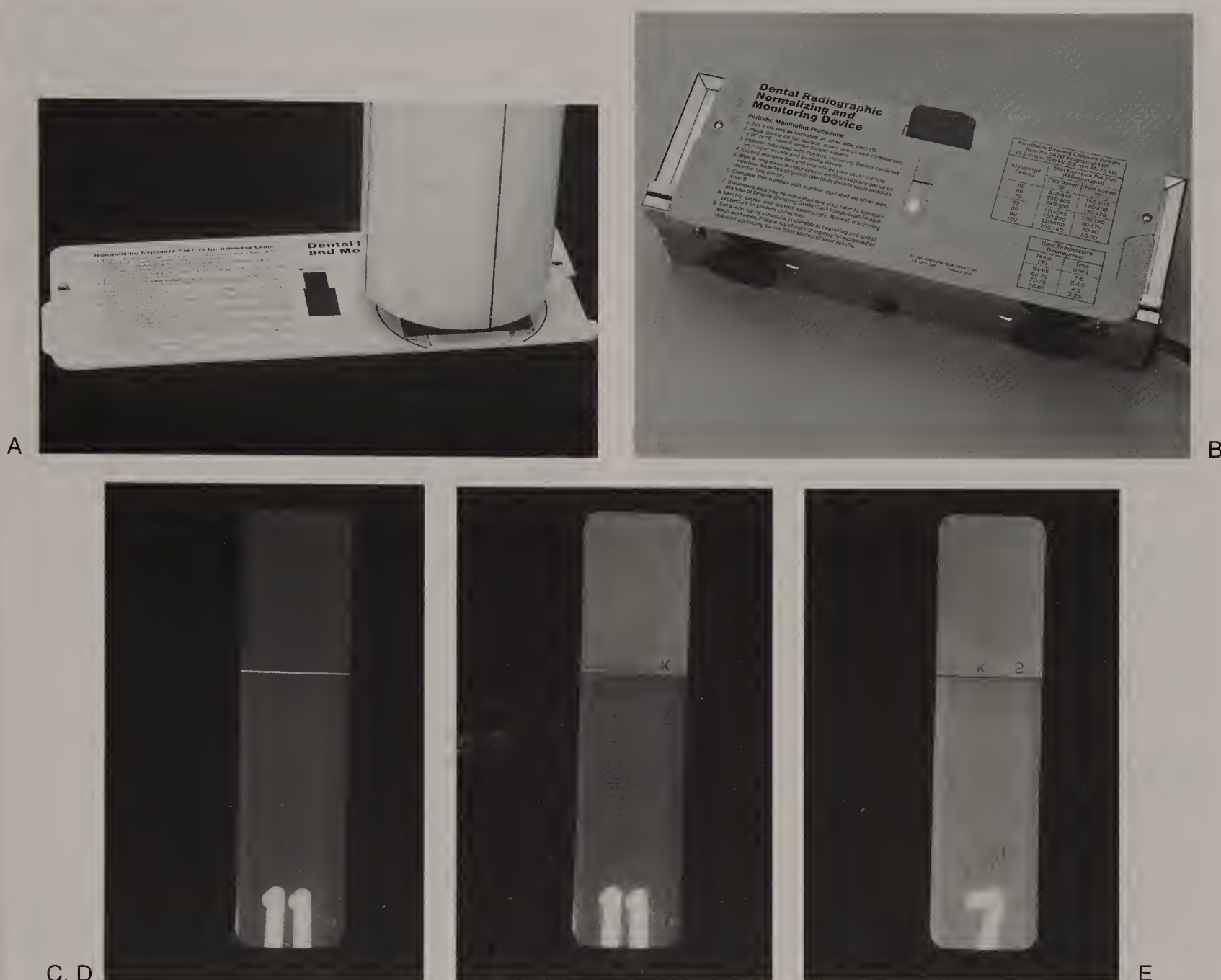
Figure 8.12 Dental Radiographic Normalizing and Monitoring Device. (A) Front of device gives instructions for exposing the monitor film. (B) The back of the device contains a slot into which the processed film is inserted and matched with the density strip. (C) Baseline monitor film measures 11 on the density strip. (D) Several days later, a newly exposed monitor film does not match the baseline reading (11). (E) By moving the density strip, a new match is found. A problem exists if the density of the monitor film changes by two or more units.
