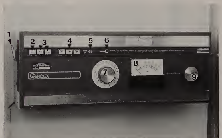
Figure 2.4 Control Panel of a Gendex Dental X-Ray Machine. (1) Holder for exposure button, (2) main switch off, (3) mA selector and main switch on, (4) x-ray tube selector, (5) power on light, (6) x-ray/emission light, (7) exposure timer, (8) kVp-mA meter, and (9) kVp selector (auto transformer).
