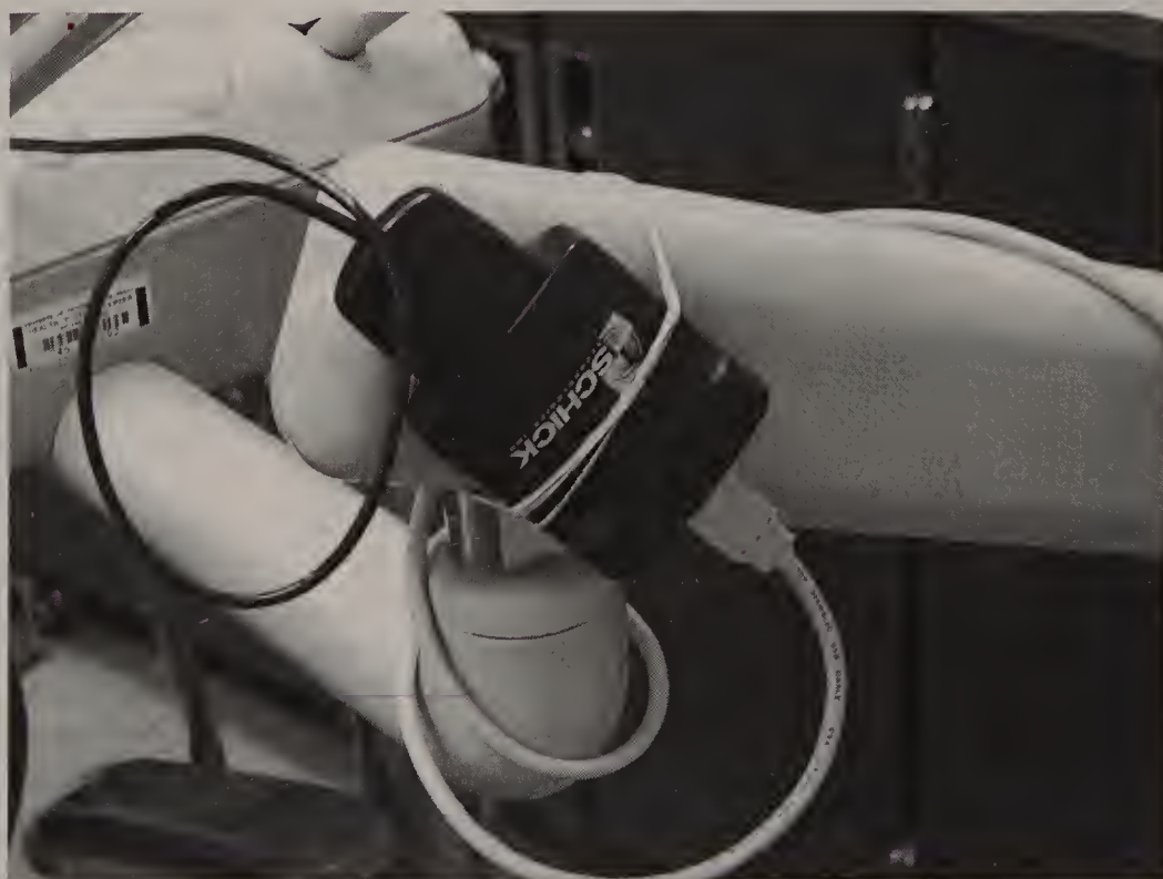
Figure 11.46 A Universal Serial Bus (USB) Connector. One major advantage of a USB connector is the low power requirement and possibility of connecting to a battery-operated laptop computer.
