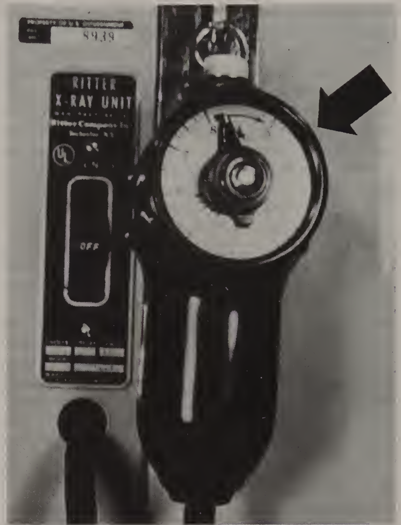
Figure 13.10 Mechanical Timers. A mechanical timer (arrow) on an older dental x-ray machine. When the button is pushed, it closes the circuit and allows the current to flow without interruption. These timers are inaccurate for exposure times shorter than 1 second.
