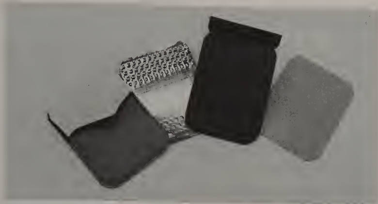
Figure 4.11 Components of Film Packet. From left to right: moisture and light-proof film packet, sheet of lead foil, black light-proof paper, and radiograph film.
