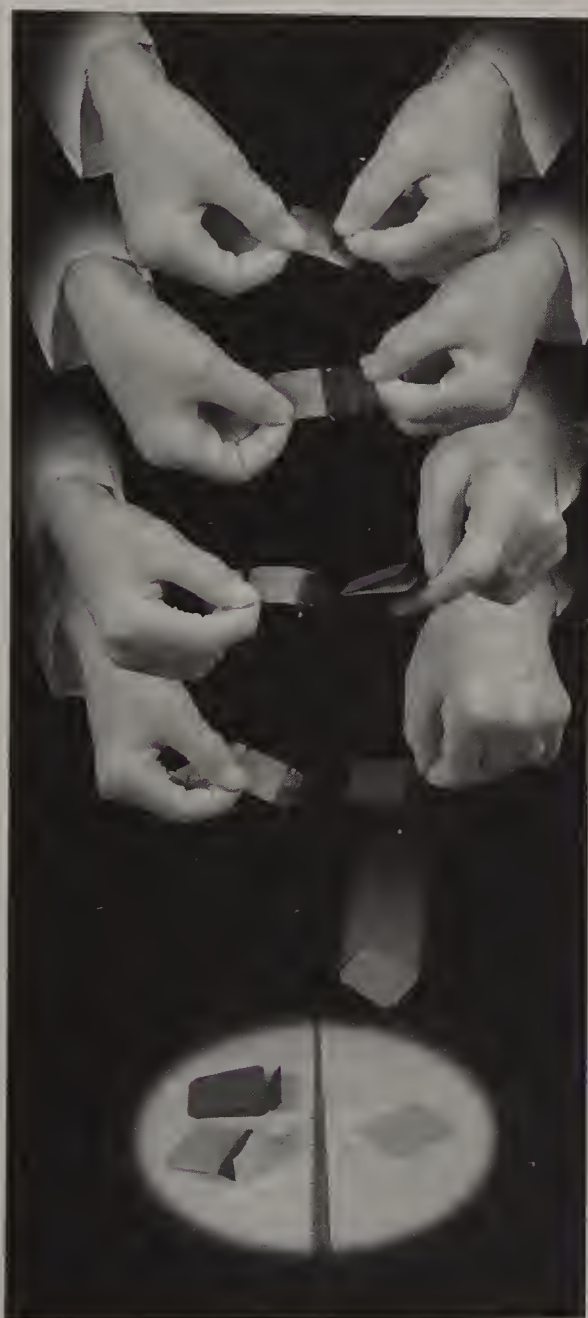
Figure 4.12 Method for Removing Films From Packet Without Touching Them With Contaminated Gloves. From top to bottom: packet tabs are grasped; packet tab is opened; black interleaf paper and film are slid from outer wrapping; and film is dropped onto clean paper towel. Contaminated film packet should be dropped onto a separate paper towel.
