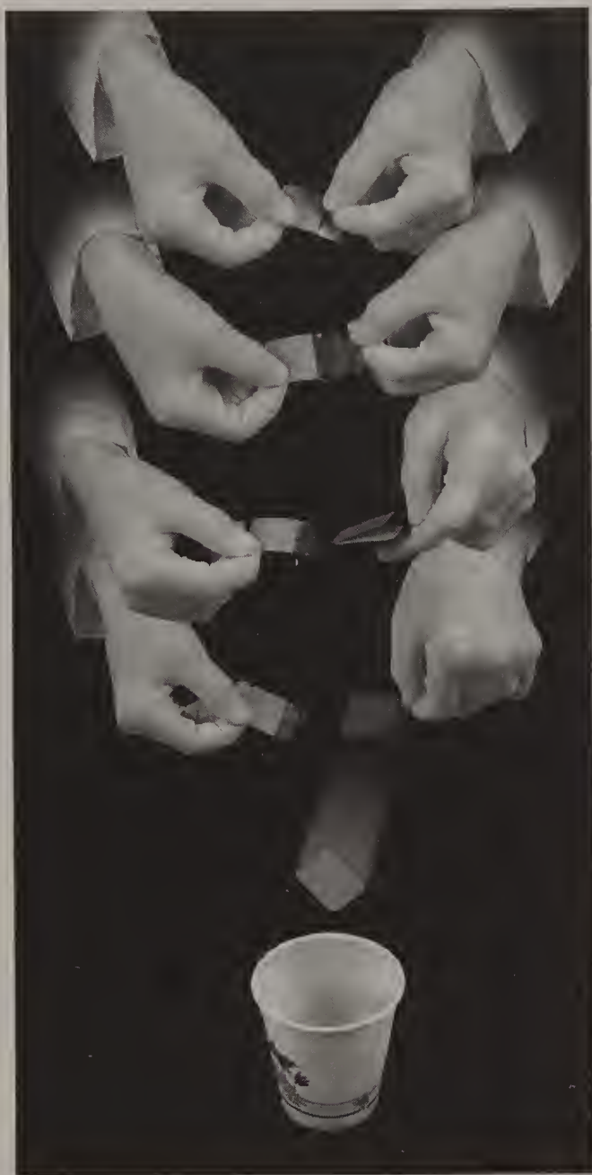
Figure 4.13 Removing Film From Packets Into Daylight Loader. With the three-glove method, powder-free latex or vinyl gloves are placed onto clean, washed hands outside the daylight loader, and the newly gloved hands are inserted through the sleeves. With powder-free latex- or vinyl-gloved hands inside the daylight loader, the polysoft cover of the film should be removed without touching the film. The film is dropped into the paper cup without being touched.
