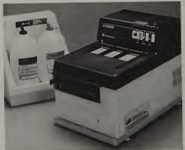
Figure 6.10 A/T 2000 Automatic X-Ray Film Processor. The A/T 2000 Automatic X-ray Film Processor automatically controls time, temperature, chemistry agitation, and chemistry replenishment. It shuts itself off as soon as the last film exits the processor and returns to a stand-by status, which saves water, electricity, and general wear and tear. Normal speed is a 5.5-minute processing cycle for archival quality dental films of all sizes up to 8 × 10 inches. Endo speed is a 2.5-minute processing cycle that provides a "quick look" for nonarchival quality periapical films used in endodontic procedures. (Courtesy of Air Techniques Inc., Hicksville, NY 11801).
