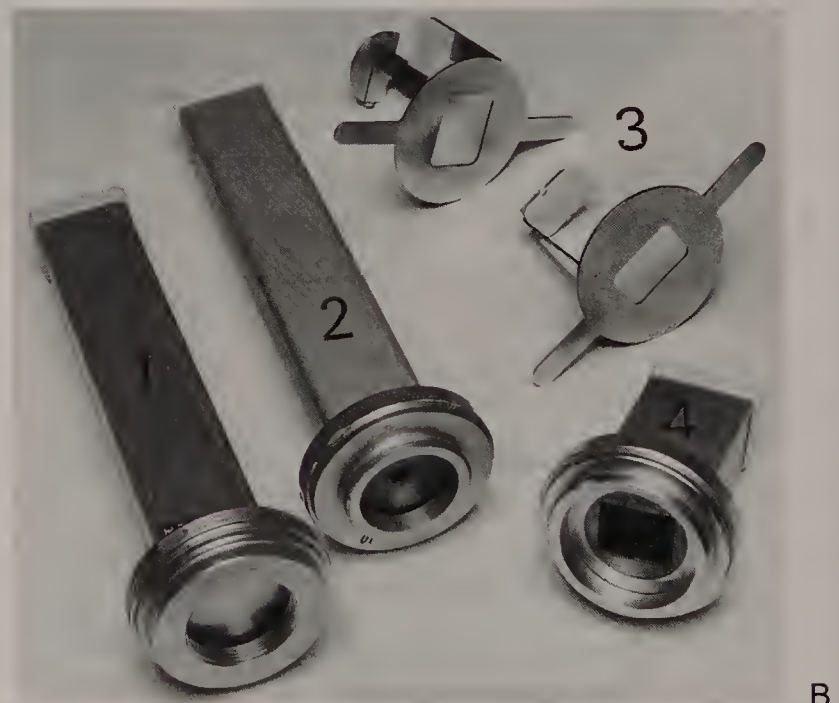
Figure 13.6 Long and Short BIDs. (A) (Above) Short and (below) long round, open-ended, lead-lined cylinders or BIDs. (B) Types of (1) rectangular collimators and (2) long Dentsply/Rinn rectangular BIDs for different x-ray machines. Rectangular BIDs are not available from Dentsply/Rinn. At present, contact Margraph Corp., 611 Harper Ave., Jenkintown, PA 19046. (3) Masel Precision Instruments (anterior and posterior instruments). (4) Rectangular BID for recessed anode tubehead.
