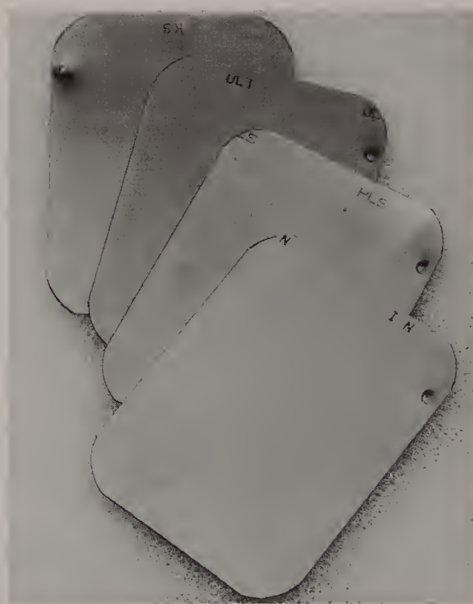
Figure 2.23 Embossed Film Markings. (A) KS: older "D" or Ultra-speed film; ULT: newer "D" or Ultra-speed film; PLS: E+ or EKTASPEED Plus film; IN: "F" or INSIGHT film. (continued)
