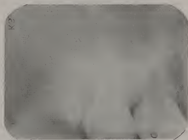
Figure 7.20 Low-Density Film. Low-density film may be the result of insufficient radiation exposure or underdevelopment of the film.
