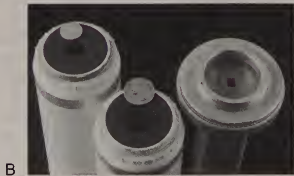
Figure 13.2 Collimation. (A) Collimation is the restriction of the cross-sectional area of the beam and is usually done with a collimator (diaphragm). A collimator can be a flat piece of lead with a round hole in it to restrict the useful beam to an area no larger than 2.5 inches in diameter when measured at the end of the BID. The size and shape of the hole in the center depends on whether the BID is short/long or rectangular/round. The collimators on the top right are for long, round BIDs (upper) and short, round BIDs (lower). (B) Collimator aperture sizes: (left) long, round BID—dime size; (middle) short, round BID—quarter size; (right) rectangular, long BID—smallest.
