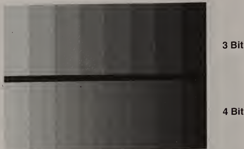
Figure 11.37 Image Quality and Gray Scale. (Top) A 3-bit image has 2 \times 2 \times 2 or 8 shades of gray. (Bottom) A 4-bit image has 2 \times 2 \times 2 \times 2 or 16 shades of gray (bottom diagram). Increasing bit depth yields more shades of gray. The human eye can see approximately 16 to 25 shades of gray.
