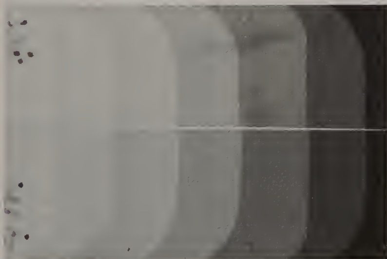
Figure 8.3 Checking Output. If the steps in the baseline image (top) match the densities of the steps in today's image (bottom), then the radiation output reading (top) has not changed between the baseline and today's reading (bottom).
